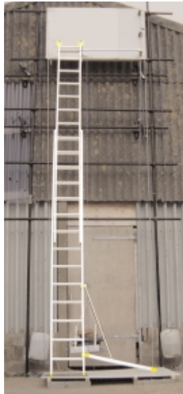
LSD actual Flip test. Ladder extended to 6.5m. Vertical Load 128kg. Horizontal Load 23kg. Stabiliser and top wheels fitted. (See overleaf).
